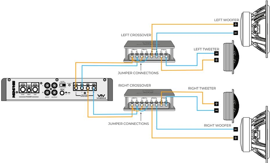
WIRING COMPONENTS - BI-AMPED SET UP
