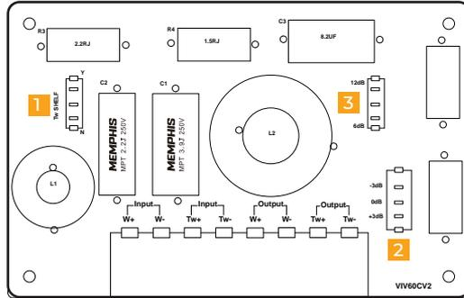
VIV60CV2 Crossovers uses switches to adjust a variety of features allowing the user to dial in the perfect sound for their audio system.
